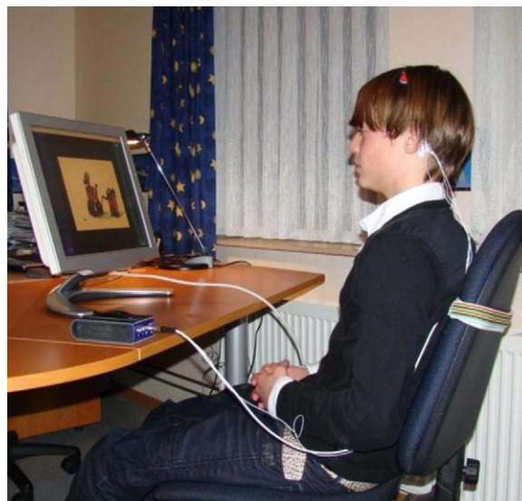
Fig. 1. Illustration of the neurofeedback setting showing a boy with electrodes at his scalp and mastoids watching the screen and trying to regulate his brain activity using the feedback to guide him.
